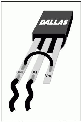
Figure 2. 1-Wire temperature sensor with V<sub>DD</sub> pin locally connected to GND.
