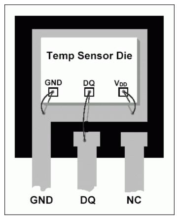
Figure 3. Cutaway view of -PAR temperature sensor.
