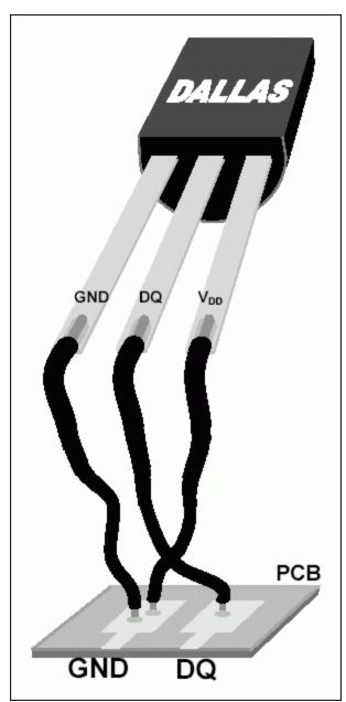
Figure 1. 1-Wire temperature sensor with V<sub>DD</sub> pin connected to GND at PCB.
