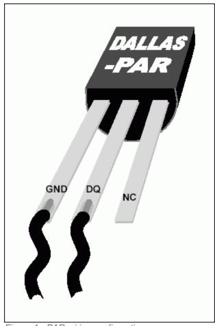
Figure 4. -PAR wiring configuration.
