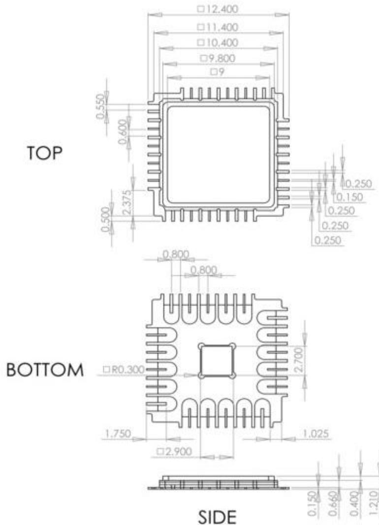
Fig. 4. 44-Pin Package Drawing (All Dimensions in mm)
