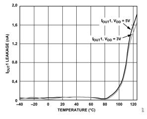
Figure 17. IOUT1 Leakage Current vs. Temperature
