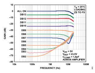
Figure 22. Reference Multiplying Bandwidth vs. Frequency and Code
