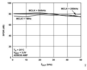
Figure 29. Wideband SFDR vs. f<sub>OUT</sub> Frequency
