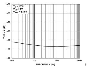
Figure 28. THD + Noise vs. Frequency
