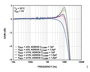
Figure 24. Reference Multiplying Bandwidth vs. Frequency and Compensation Capacitor
