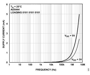
Figure 20. Supply Current vs. Update Rate
