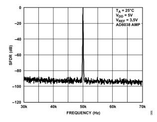
Figure 33. Narrow-Band SFDR, f<sub>OUT</sub> = 50 kHz, Clock = 1 MHz
