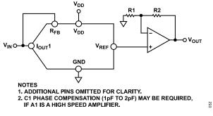
Figure 40. Single-Supply Voltage Switching Mode Operation
