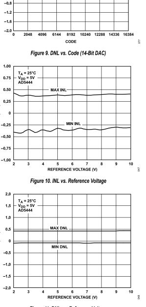
Figure 11. DNL vs. Reference Voltage
