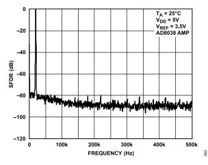
Figure 30. Wideband SFDR, f<sub>OUT</sub> = 20 kHz, Clock = 1 MHz
