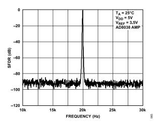
Figure 32. Narrow-Band SFDR, f<sub>OUT</sub> = 20 kHz, Clock = 1 MHz
