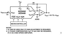
Figure 38. Unipolar Operation
