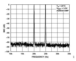
Figure 34. Narrow-Band IMD, four = 20 kHz and 25 kHz, Clock = 1 MHz
