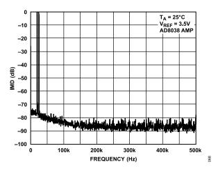
Figure 35. Wideband IMD, f<sub>OUT</sub> = 20 kHz and 25 kHz, Clock = 1 MHz
