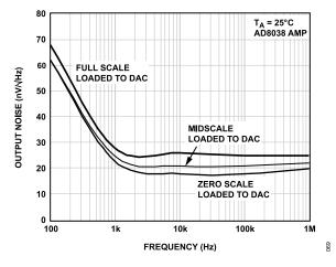
Figure 36. Output Noise Spectral Density
