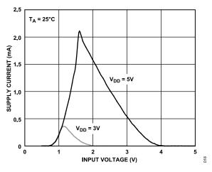
Figure 18. Supply Current vs. Logic Input Voltage
