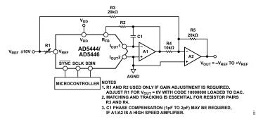
Figure 39. Bipolar Operation (4-Quadrant Multiplication)
