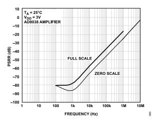
Figure 27. Power Supply Rejection Ratio vs. Frequency
