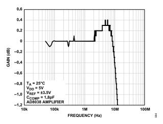
Figure 23. Reference Multiplying Bandwidth vs. Frequency—All 1s Loaded
