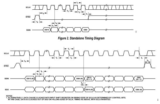
Figure 3. Daisy-Chain Timing Diagram
