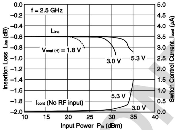
**RFC-RF1/RF2  $P_{in}$  (0.1 dB) vs. INPUT POWER**
