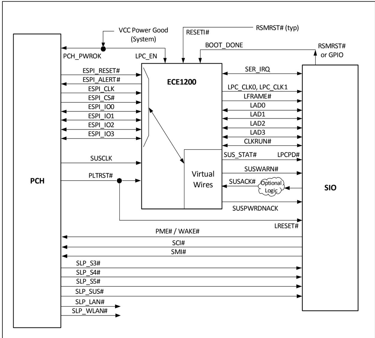
**Note 1:** SMI# can instead be presented on SER\_IRQ pin (time slot 2) and propagated to the PCH as a Virtual Wire.
