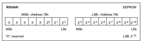
Figure 1. The calculated RSGAIN value should be written to addresses 78h and 79h using the above RSGAIN Register format.
