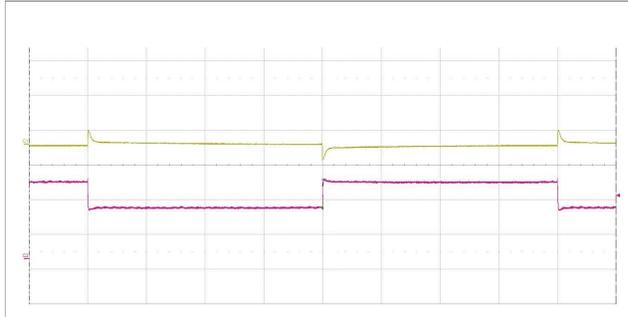
Output voltage response to load current step-
