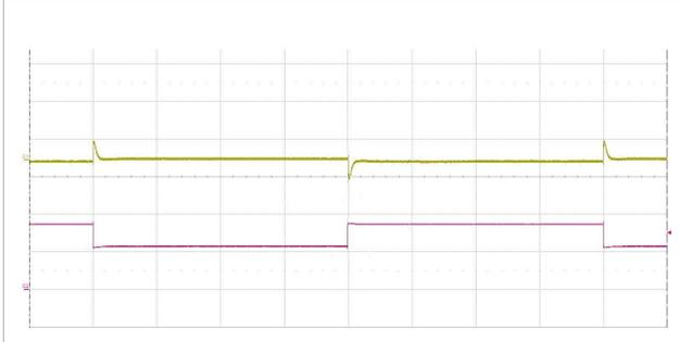
Output voltage response to load current step-
