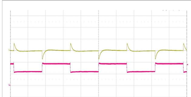
Output voltage response to load current step-
