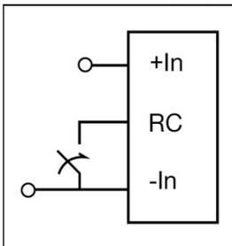
The products are fitted with a remote control function referenced to the primary negative input connection (-In), with negative and positive logic options available. The RC function allows the product to be turned on/off by an external device like a semiconductor or mechanical switch. The RC pin has an internal pull up resistor to +In.
