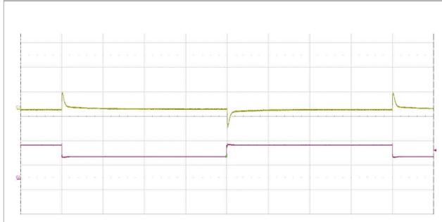
Output voltage response to load current step-
