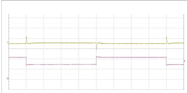
Output voltage response to load current step-change (3.0-4.5-3.0 A) at:
