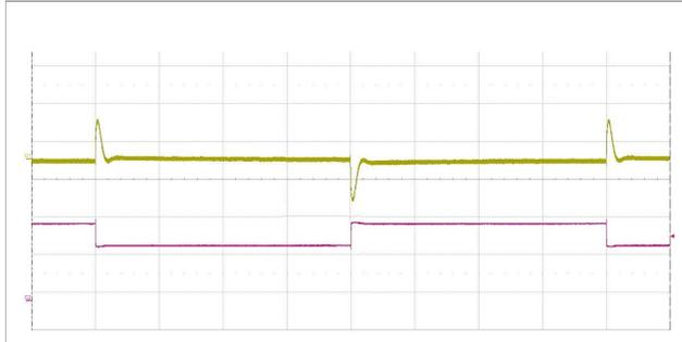
Output voltage response to load current step-
