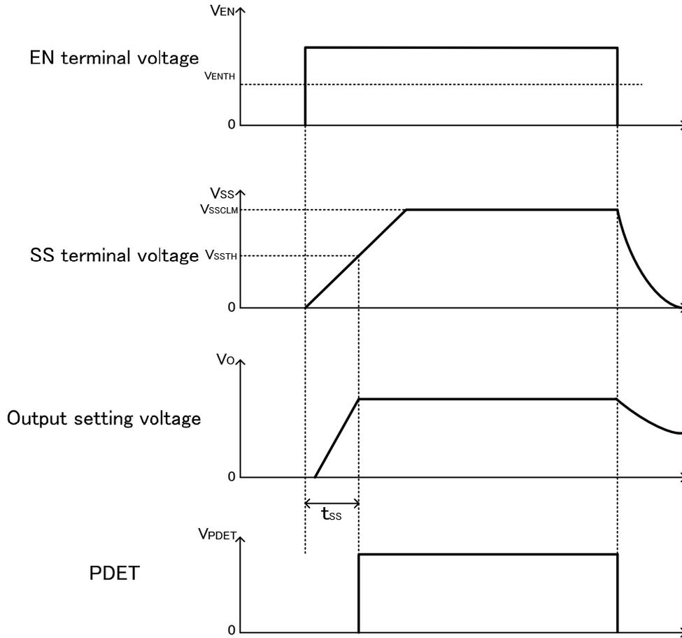
**Fig. 3 ON/OFF transition wave form in EN controlling**
