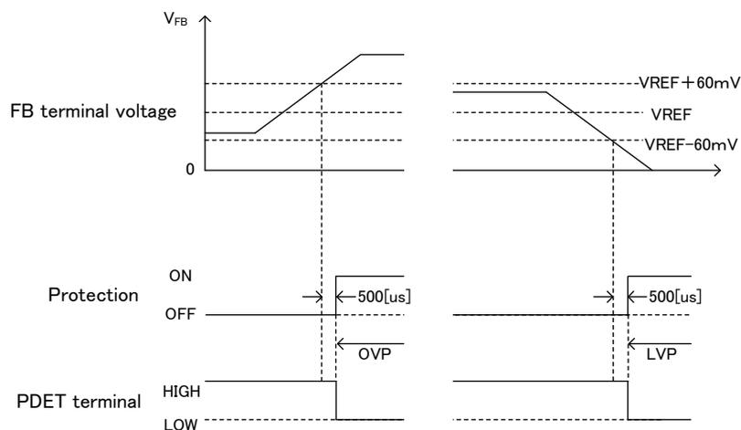
Fig. 5 Output voltage error detection range
