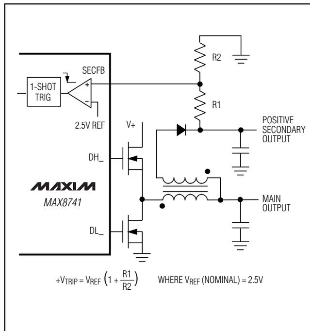
Figure 5. Adjusting the Secondary Output Voltage with SECFB
