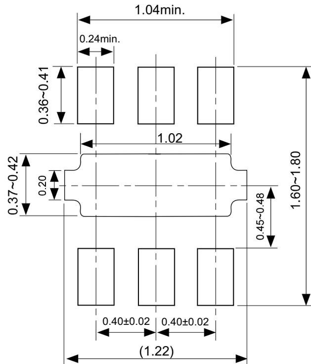
Caution It is recommended to solder the heat sink to a board in order to ensure the heat radiation.
