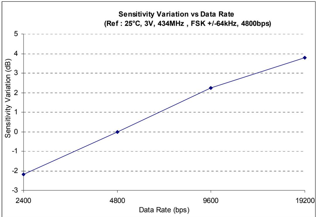
**Figure 39. FSK Sensitivity Variation Versus Data Rate**
