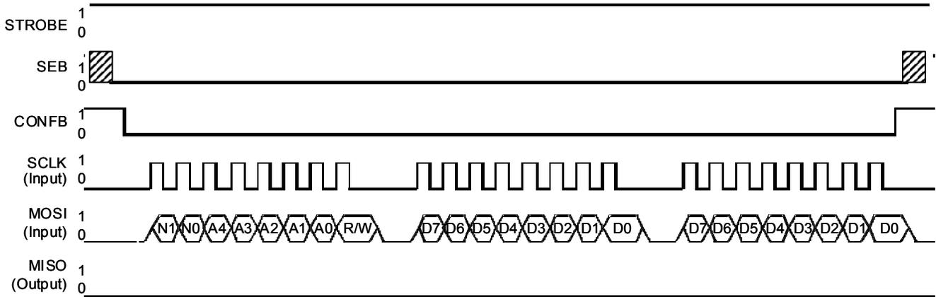
**Figure 19. Write Operation in Configuration Mode (N[1:0] = 01)**
