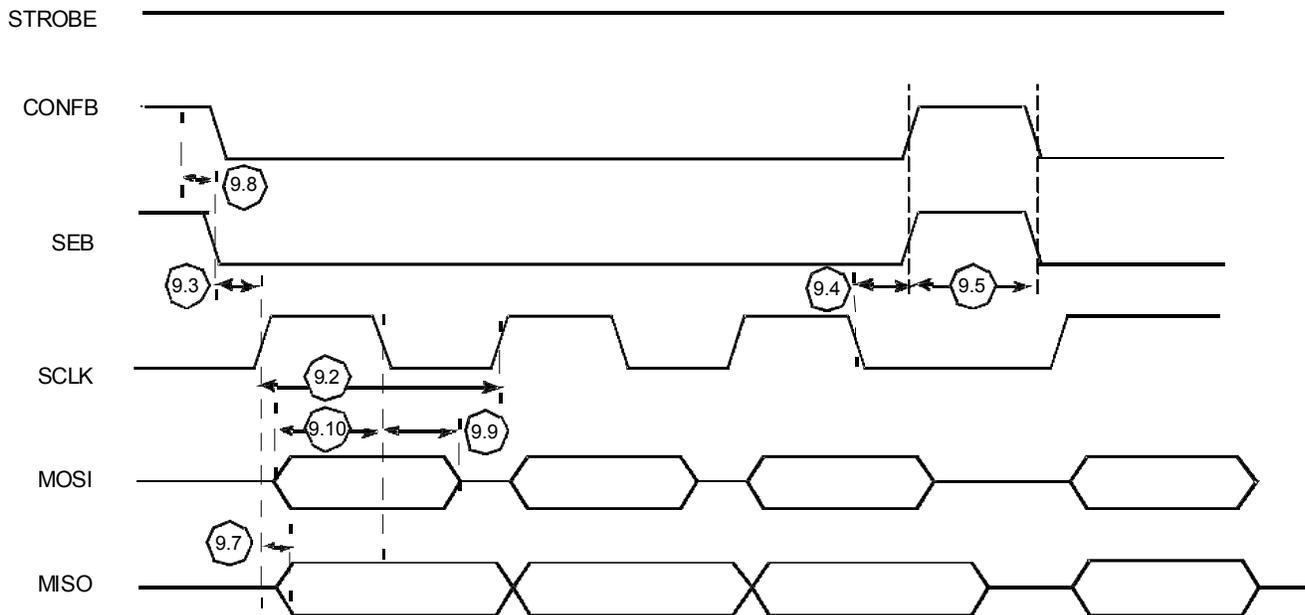
Figure 41. Digital Interface Timing Diagram in Configuration Mode
