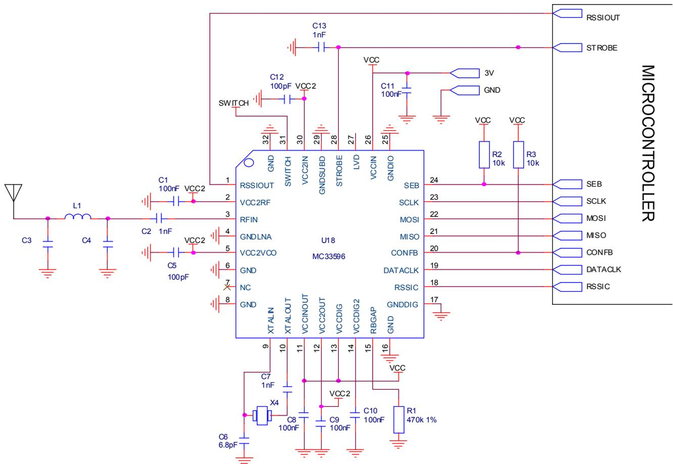
Figure 44. MC33596 Application Schematic in Strobe mode (3 V)
