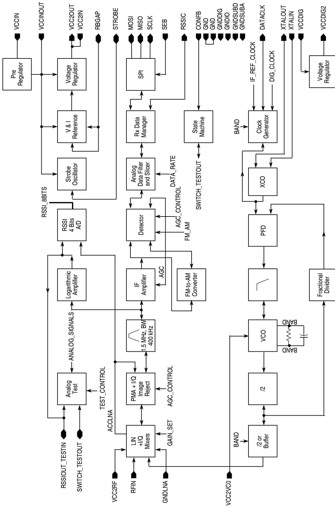
Figure 1. Block Diagram
