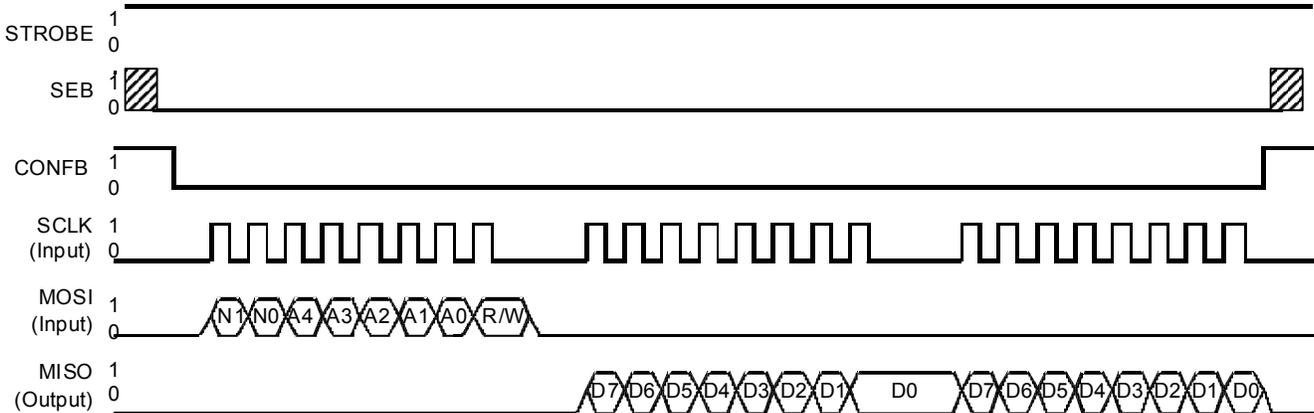
**Figure 20. Read Operation in Configuration Mode (N[1:0] = 01)**
