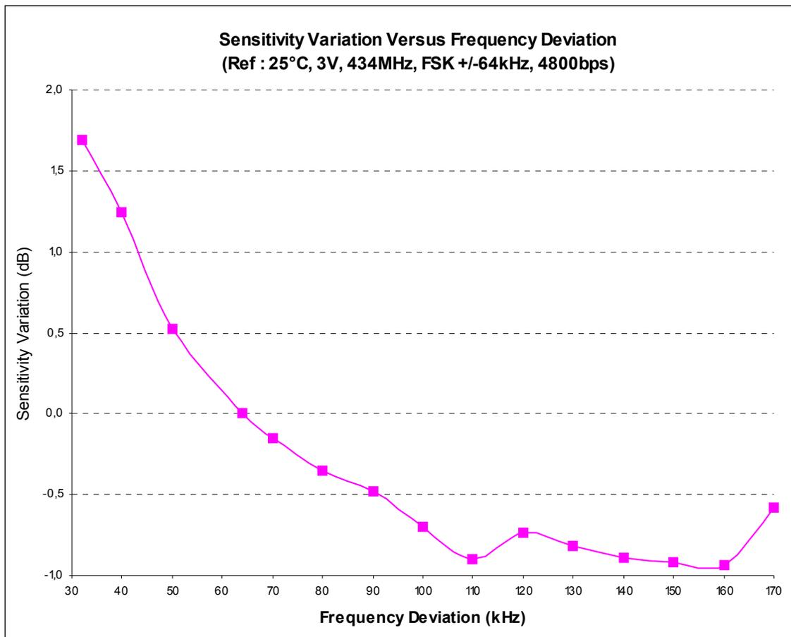
Figure 40. FSK Sensitivity Variation Versus Frequency Deviation
