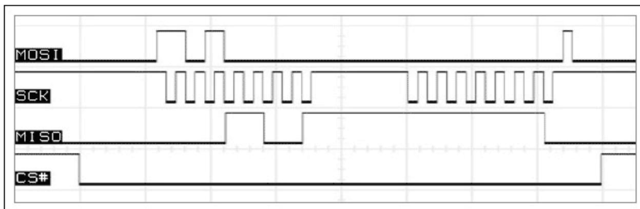
Figure 5. SPI interface operating in mode (1,1).
