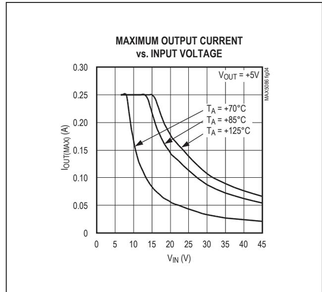
Figure 4. Maximum Output Current vs. Input Voltage
