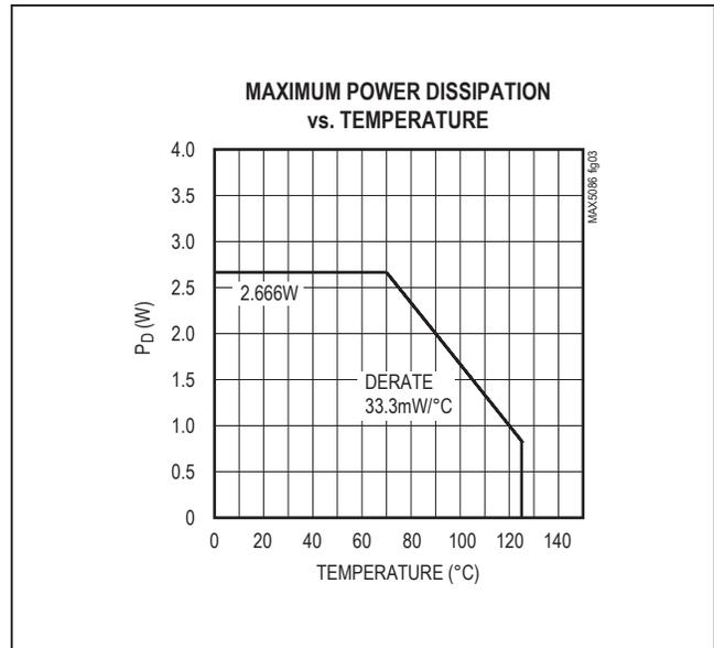
Figure 3. Calculated Maximum Power Dissipation vs. Temperature
