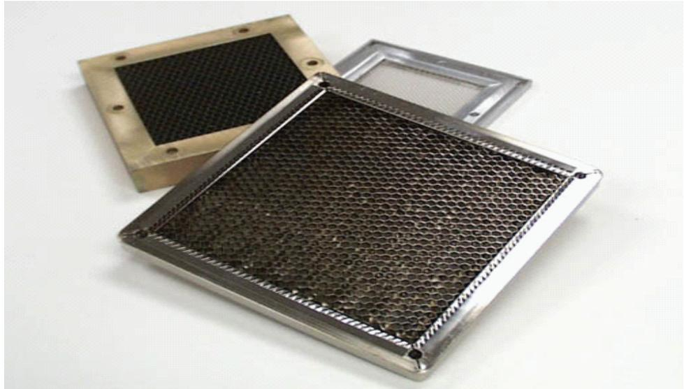
For improved shielding effectiveness and environmental protection, these lightweight aluminum ventilation panels are available tin plated. However, in applications requiring maximum shielding levels and greater weight support, either steel or brass honeycomb shielded vents are recommended. (Refer to page 164, Steel and Brass Honeycomb Shielded Vents, for specifications.)
