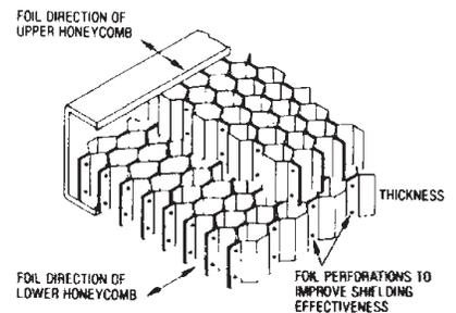
Figure 1 OMNI CELL Honeycomb Construction
