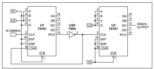
Figure 2. Synchronous counters can divide by any integral multiple of the input. Here, division by 6, then by 8, divides the input by a factor of 48.
