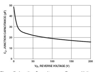
Figure 7. Junction Capacitance vs Reverse Voltage
