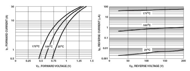
Figure 1. Forward Current vs Forward Voltage
