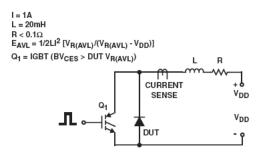
FIGURE 10. AVALANCHE ENERGY TEST CIRCUIT
