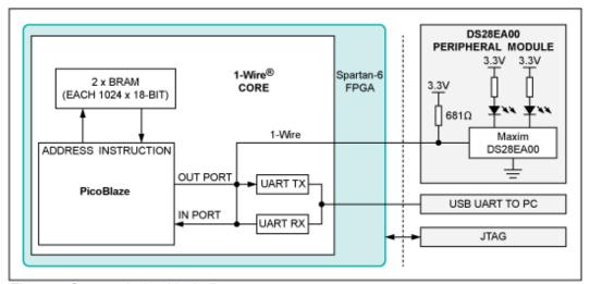
Figure 1. System design block diagram.
