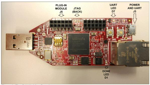
Figure 2. The S6LX9 MicroBoard.
