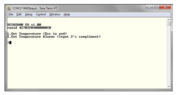
**Note**: If the "romid" shows all zeroes, recheck your connections. The DS28EA00 peripheral module likely does not have correct orientation or is plugged into the wrong row.
