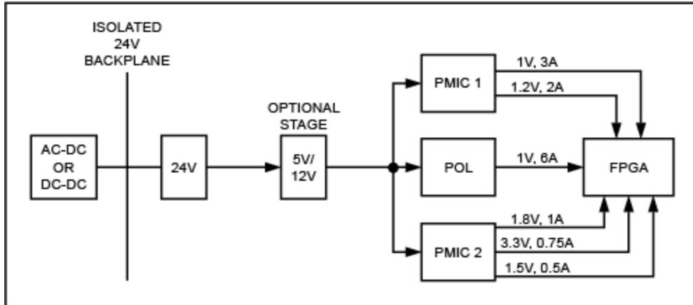
Figure 1. A simplified block diagram shows the power architecture in industrial FPGA applications.
